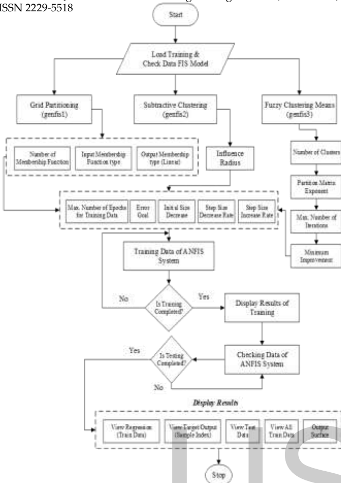
Fig. 5. Proposed Block Diagram of ANFIS-AOLM Training Model
